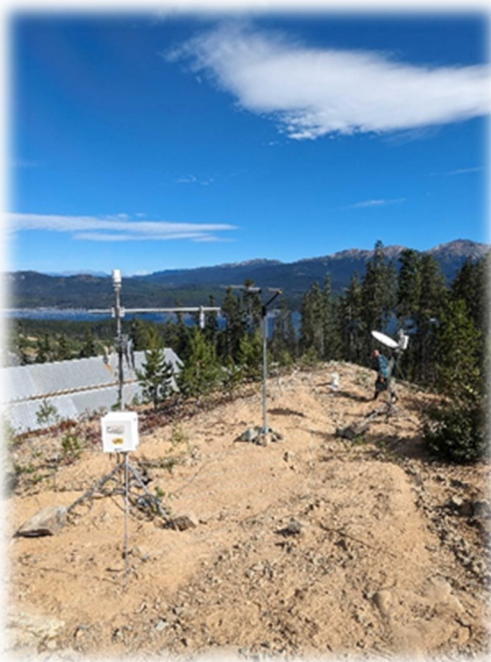
Figure 12: Meteorological station, Parsivel, and MRR deployed at Huckleberry Mines.
