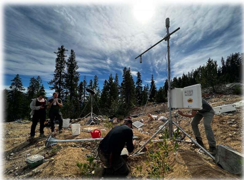
Figure 7: NHG field crew setting up meteorological station at Huckleberry Mines, Upper Nechako.
