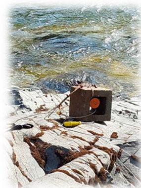
Figure 21: Logger in a PVC pipe that is secured to a cinderblock and tethered to an anchor.
