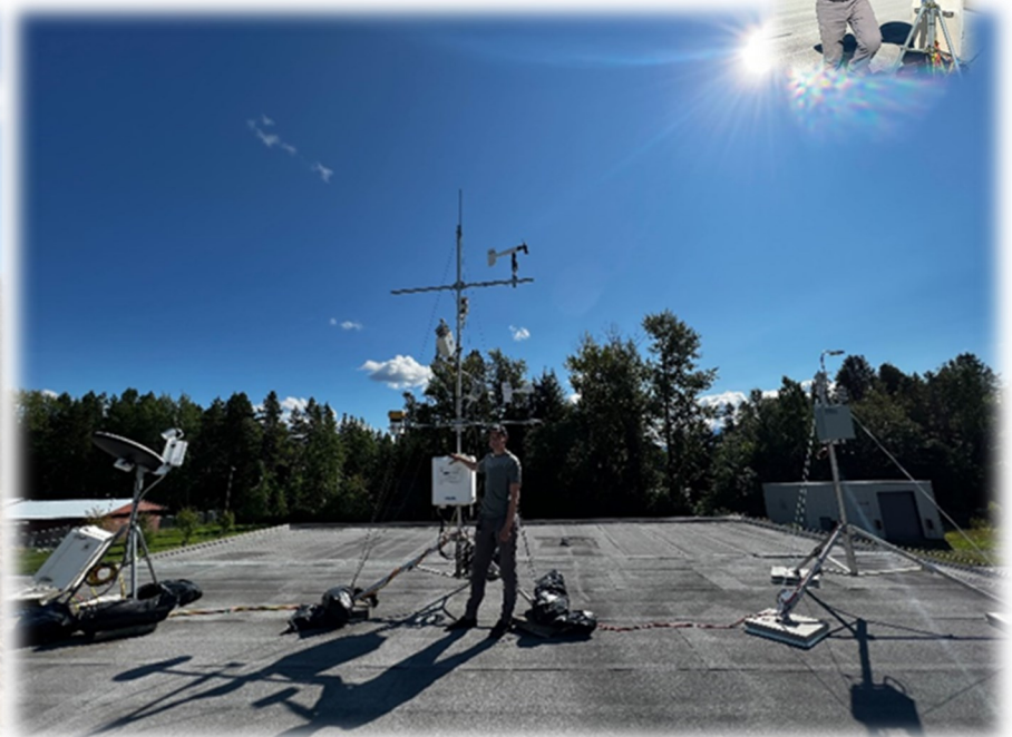
Figure 13: Terrace roof top set-up, including Hotplate, icing detector, MRR, and meteorological station.
