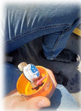
Figure 20: MX2201 blue-tooth logger with equipment code sticker.
