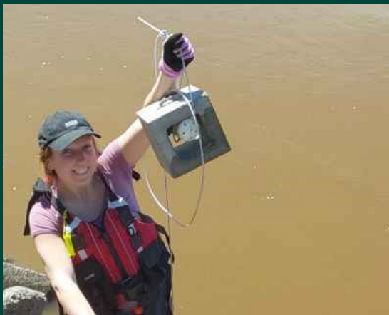
Above: Jade retrieving a stream temperature probe
