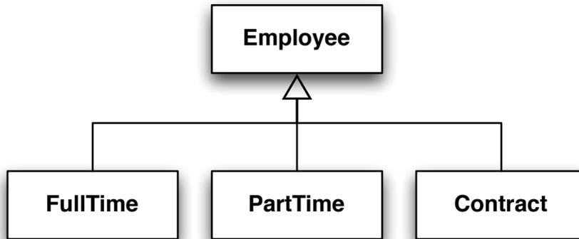
Figure 1: Inheritance Diagram
