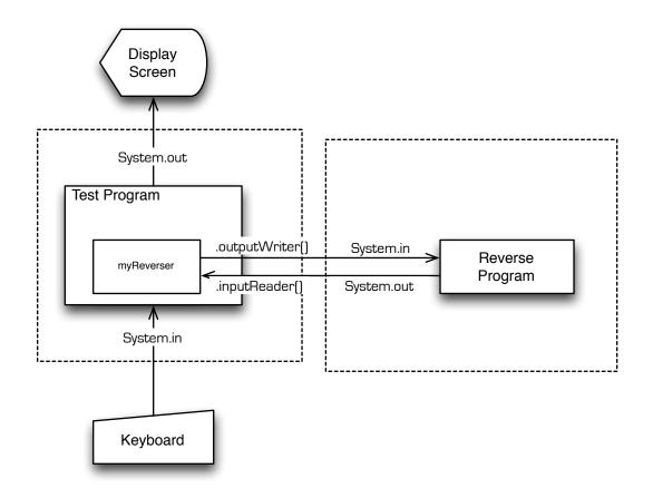
Figure 1: Illustration of a program using JavaPipe
