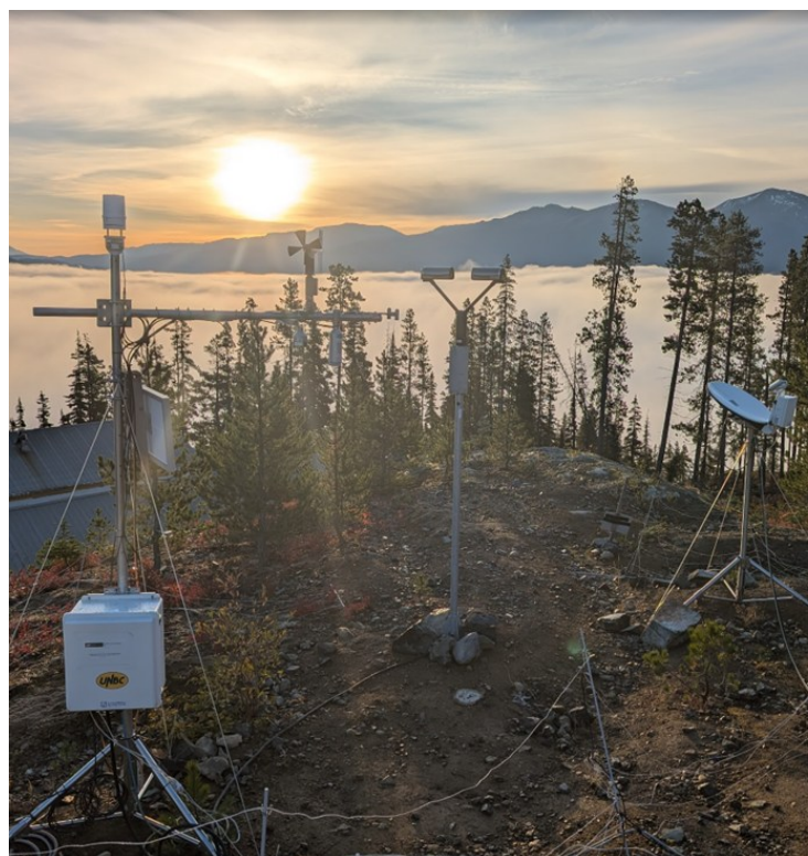
Figure 8. Huckleberry Mine. Left to Right: Weather Station, Parsivel Disdrometer, Micro Rain Radar.
