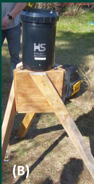
Figure 2: (A) Weather station build during training session, (B) tipping bucket rain gauge, and (C) water temperature logger system.
