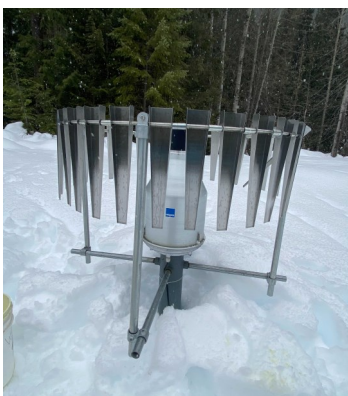
Left: The Geonor all-weather precipitation gauge at QRRC, 15 February
