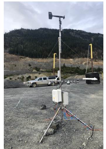
Images: (Top) Huckleberry Mine storm monitoring equipment. (Bottom, left to right) Pond Hotplate Weather Sensor, Metek Micro-Rain Radar, OTT Parsivel Laser Disdrometer, Weather station with wind speed, net radiation, air temperature and relative humidity.
