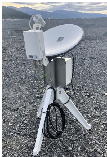
Images: (Top) Huckleberry Mine storm monitoring equipment. (Bottom, left to right) Pond Hotplate Weather Sensor, Metek Micro-Rain Radar, OTT Parsivel Laser Disdrometer, Weather station with wind speed, net radiation, air temperature and relative humidity.
