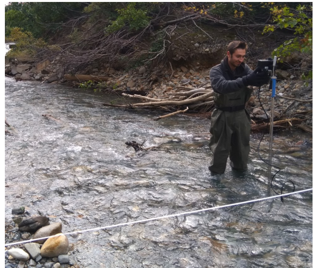
Images: Stream velocity measurements, by Anna Kaveney in Rhine Creek (top) and Emile Cardinal in Whiting Creek (bottom).
