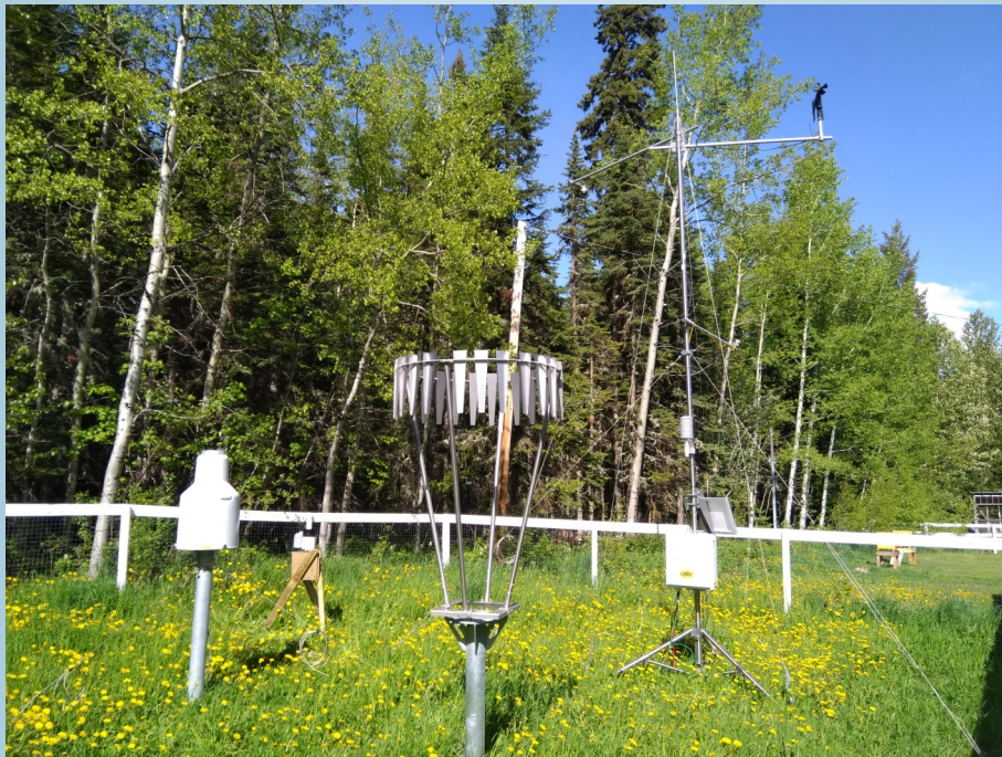
Figure 2. Future Mt Sweeney weather station under going testing in the Research Manager's back yard. The station consists of a 6 m tripod with snow depth, wind, solar radiation and atmospheric pressure sensors, and a Pluvio2 weighing precipitation gauge (cone shaped sensor in photo). Once the Pluvio2 is installed at Mt. Sweeney, it will be mounted at a height of 3 m within the windshield pictured in the foreground. Hiding at the back left of the photo is one of the 10 tipping bucket rain gauges to be deployed across the reservoir region.
