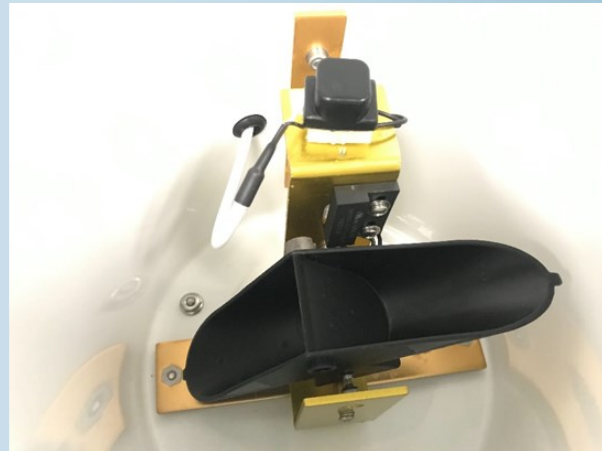
Figure 3. Tipping mechanism within the tipping bucket
