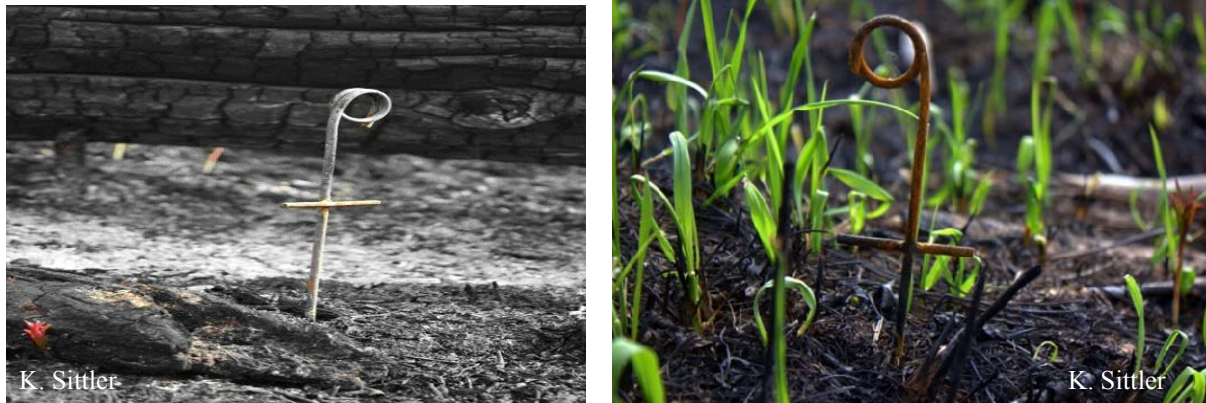
Figure 5. Depths of burn pins were used to measure the amount of fuel consumed as an index of the intensity of a burn.
