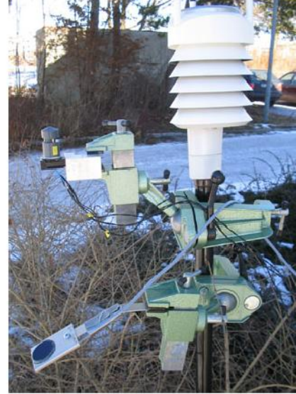
Fig. 14. View of the weather sensor consisting of a simple Pt100-resistor attached below a water absorbent foam surface (above) and general view of the sensor arrangement with reference sensor (Vaisala WTX50)
