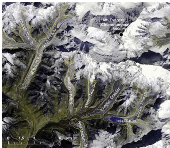
Figure 5. Automatically delineated areas of debris-covered glaciers (yellow polygons) based on ASTER.
