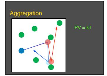
What can be done? If this were a simple gas, the over-all behaviour can be approximated by this equation: pressure times volume is proportional to temperature. Note that these variables are aggregate properties, they do not exist at the molecular level. Pressure and temperature are related to mean and mean-square speeds.
