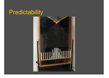
An apparatus sometimes used in probability demonstrations. Ball-bearing balls drop through an arrangement of pins, into bins at the bottom. Trying to predict the fate of any of the individual balls is hopeless. But we can predict reasonably well their average final positions, and to some extent, their variance. With a large enough sample, we can also have some idea of the distribution.
